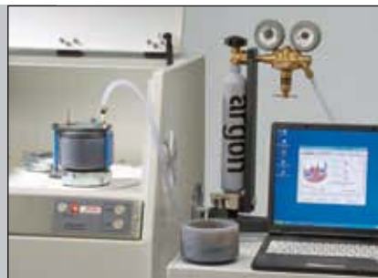
The PULVERISETTE 4 grinding in inert gas
