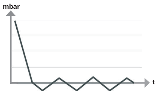
Schematic view of two-position vacuum control
