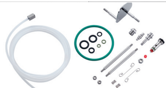
C 6000.10 Set of spare parts For C 6000 calorimeter and C 6010 decomposition vessel; includes various o-rings and seals; a ventilation hose with capillary; two ignition and ground electrodes; 10 ignition wires; a complete piston; a nozzle; two compression springs; spare Hastelloy nuts Ident. No. 0004504300
