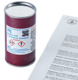
C 43 Benzoic acid NBS 39i High pure benzoic acid powder; 30 g; standard reference material with certificate of the National Institute of Standards & Technology (NIST), USA Ident. No. 0000750600
