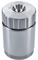
C 7012 Decomposition vessel, halogen resistant Material: halogen resistant stainless steel with catalytic activated inner surface. Especially for combustion / decomposition of halogen and sulfur containing samples Ident. No. 0003017000
