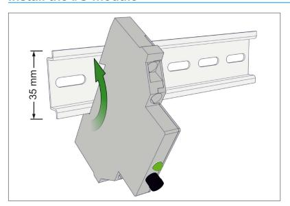
⇒ Clip the I/O module onto a 35 mm hat rail, e. g., inside a switch cabinet or a distribution box.
