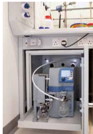
Chemical network pumping unit under the exhaust hood, with solvent recovery
