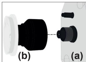
1. Remove the blind plug and place the small flange KF DN 16 **(b)** on the vacuum connection of the sensor **(a)**.
