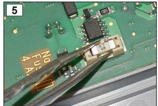
5. Insert the new fuse into the base.
