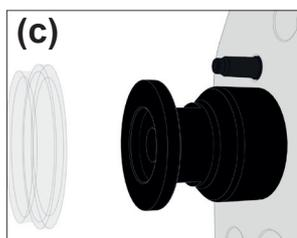
3. Remove the protective dust cap **(c)**.
