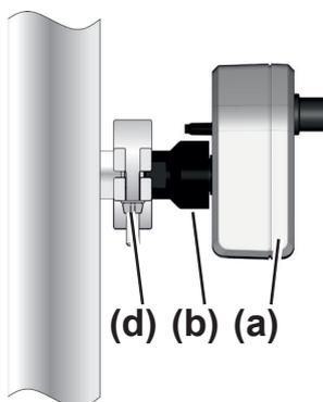
4. Place the sensor with the centering ring on the connection of the equipment → small flange KF DN 16 **(b)**.
