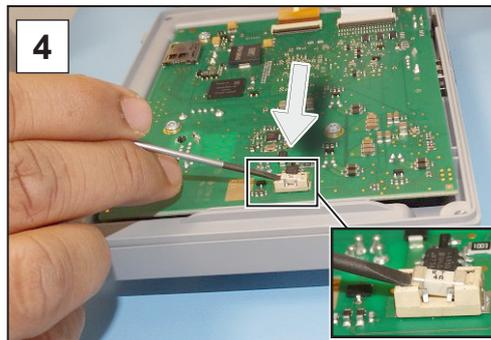
4. Lever the fuse out of the base.
