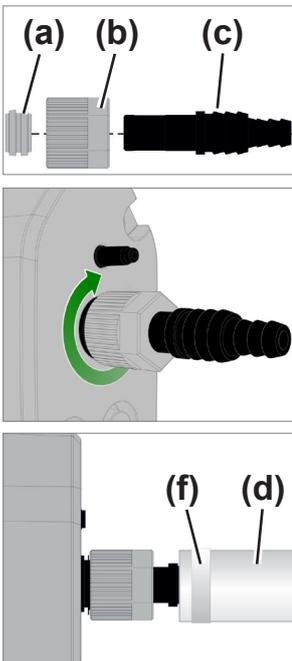
**Required connection material:** Hose nozzle DN 6/10 mm, union nut M14x1, sealing ring; optional: vacuum hose and appropriate hose clip.
