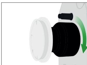
2. Tighten the small flange KF DN 16 until hand-tight.
