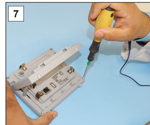
7. Tighten the housing screws with the Torx screwdriver; torque 1.1 Nm.
