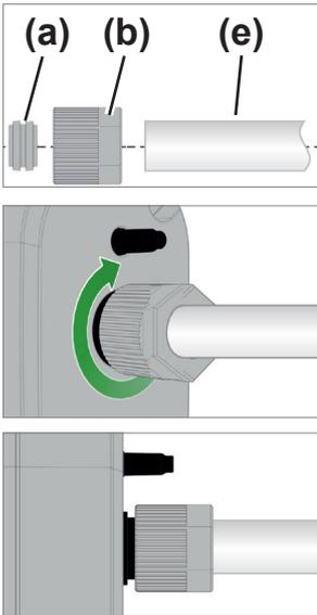
**Required connection material:** Union nut M14x1, sealing ring, PTFE hose.
