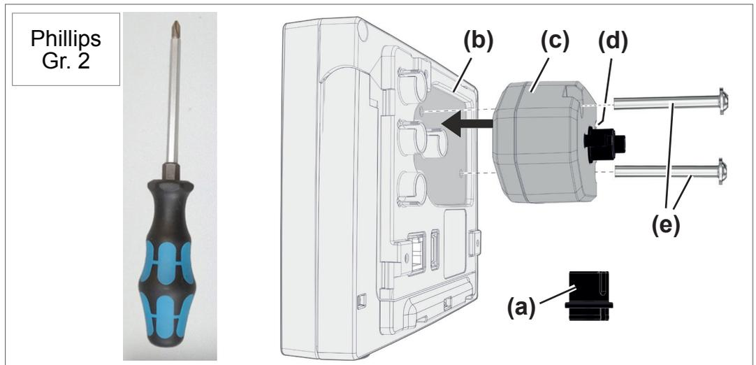
1. Pull out the VACUU-BUS® plug attachment (a) and insert it into (d).
