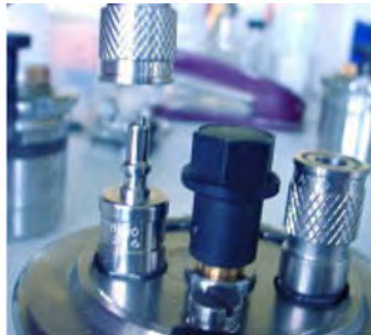
a Quick-release coupling structure with screwed pipe fitting
