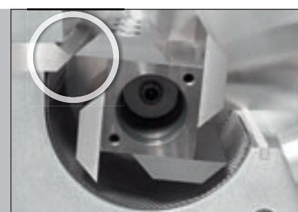
Powerful PULVERISETTE 15 cutting rotor with 4 straight cutting edges
