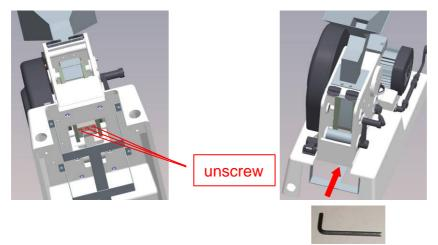
To replace the movable crushing plate (22), pull the collecting vessel (12) out of its mount. The screws of the clamping block (24) are now accessible without removing the movable crusher jaw (21). **Loosen** the clamping block (24) and lift out the crushing plate (22). Insert the new plate (or the old turned one) from below and fasten it to the clamping block (24), which must then be screwed in tightly.
