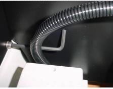
1. Loosen the lower hex socket screws (b) of the rear cover (26) with the provided Allen key a). Only unscrew these two screws one turn. The two upper screws must be unscrewed entirely.
