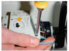
9. Loosen and remove the blue cable link (X) with a Phillips screwdriver.
