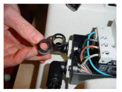
8. Position the mains cable (5) vertically and screw in the angled screw coupling (B or D). Because there is very little space here for screwing, it may be necessary to move the mains cable (5). Screw in the angled screw coupling (B or D) firmly until it stands vertically. Then press the removed collar back onto the coupling.
