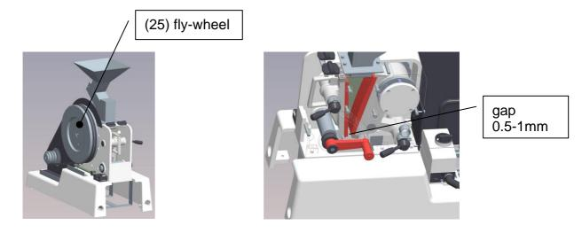
After installing the crushing plates (18, 22), you must check the gap between the plates:
