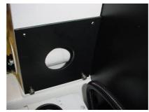
2. Pull up the rear cover (26) and slide the cover dust extraction (27) with the oblong holes onto the screws. Make certain that the washers are positioned under the screw heads. Screw in both upper screws and retighten the lower screws.
