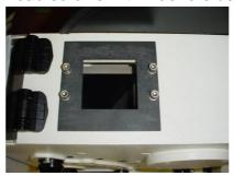
3. Pull the rubber seal over the funnel neck. Take note of the positions of the holes in the filling funnel and rubber seal.
