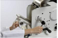
In order to access the grinding chamber, first remove the fixed crushing jaw (15), therefore open the front cover (10). The actual dismantling: Pull the guide bolt (3) off and lift the crushing jaw (15) in an upward motion.
