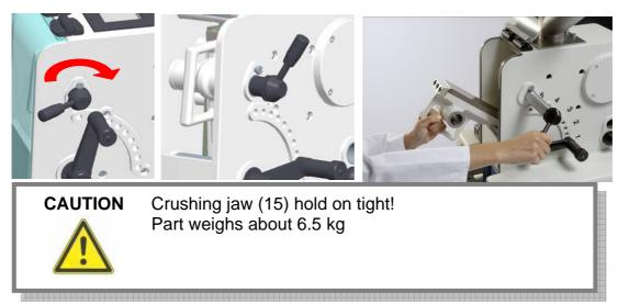
To replace the **fixed** crushing plate (18), remove the guide bolt (3) and take out the crusher jaw (15).
