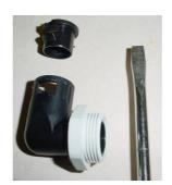
4. Then press the collar piece out of the angled screw coupling (B or D) as shown above.
