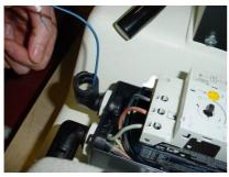
10. Then run the cable of the safety switch of the funnel (A) into the angled screw coupling (B or D) and into the housing.
