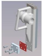
You can adjust the gap by removing or adding a compensating plate (20) under the pressure plate (19) on the fixed crusher jaw (17).
