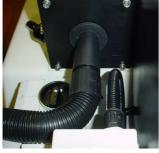
5. Then insert the reducing adapter (d) into the rubber collar (f) of the cover dust extraction (27).
