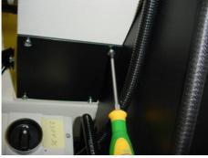
13. Fasten the cable conduit of the funnel (A) to the rear cover (26) of the jaw crusher. To do this, remove the screw on the upper right with a Phillips screwdriver (N).
