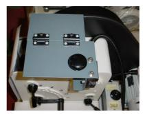
2. Mount the funnel (A) in the position shown above with the 4 cylinder head screws M6x12 (E) and the 4 washers (F).
