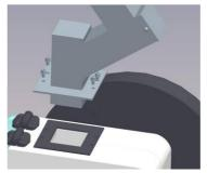
1. Remove the filling funnel (1) by unscrewing the 4 cylinder head screws using the supplied Allen key (a). Please store the screws and washers with the filling funnel (1) for subsequent reinstallation. The rubber seal remains on the housing.
