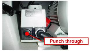
6. Use a sharp object (Phillips screwdriver) to punch through the housing of the main switch (4) in the threaded hole for the angled screw coupling so that the cable of the funnel (A) can be run through.
