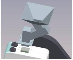
5. Screw the filling funnel onto the housing with the 4 previously removed cylinder head screws and washers.
