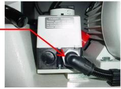
3. Select the angled screw coupling (B or D) with the correct thread (PG11 or M20). To do this, check the housing of the main switch (4) to see which thread matches.
