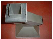
4. Insert the filling funnel into the funnel opening on the top of the laboratory jaw crusher.
