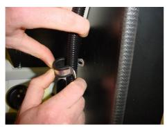
14. Slide the cable clamp (H) onto the funnel cable.
