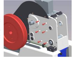
The fastening screws of the other support wall can be directly reached. After having unscrewed them, the support wall can also be removed from the inside.
