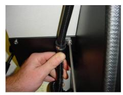
15. Then screw on the cable clamp (H) at this position with the cylinder head screw M6x12 (G).
