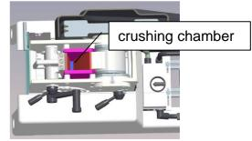
The feed rate depends on the crushing behaviour of the material. For each new material observe the crushing (crushing noise) and determine the optimum amount of material.
