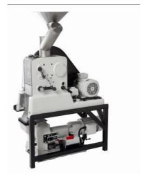
Coarse material can be comminuted to the fineness of the disk mill in one pass by combining it with the disk mill "pulverisette 13".
