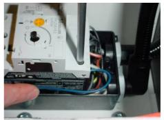
11. Screw on the short brown cable on the upper left and the long blue cable on the lower right (where the blue cable link (X) was previously connected).
