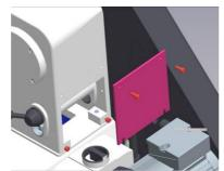
Loosen the 4 screws of the cover on the back of the grinding chamber (26 or 27 see chapter 6.1). Remove the cover and vacuum the hollow area behind it.
