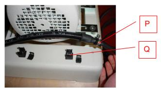
7. Open the clip (Q) of the mains cable (5) and screw off the cable clamps (P).
