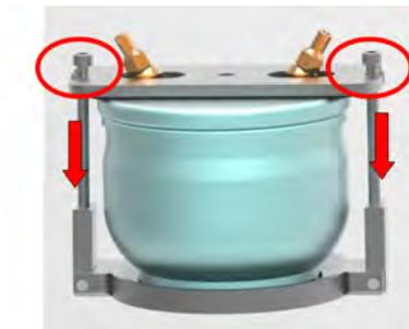
4. → Then secure the pressure plate on both sides with the socket-head screws shown in the picture and a hex key.
