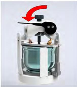
6. → Then press the clamping lever downwards. Re-tighten the additional clamping system with a hex key. The additional clamping system may be loosened due to the clamping of the Safe-Lock using the clamping lever.
