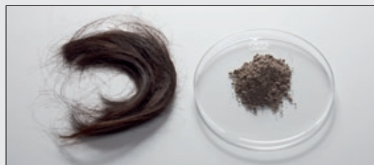
Hair sample before and after grinding with the FRITSCH PULVERISETTE 23
