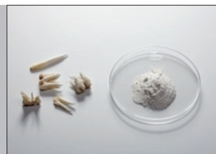
Teeth before and after grinding with the FRITSCH PULVERISETTE 0
