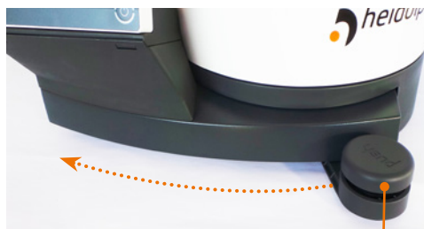
Manual lift lever: Lift position top
