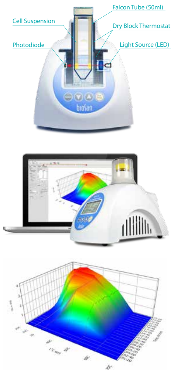
Figure 1. 3D graph of E.coli BL21 growth kinetics showing the effect of different temperatures in 7 parallel RTS bioreactors.
