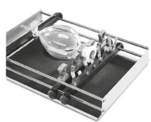
The cramp strips and spring strips are necessary for fastening separating funnels. The necks of the separating funnels are fastened in the grey plastic clamps, the spring strip secures the stoppers. The stems of the separating funnels are placed on a clamping strip h. For a modification
