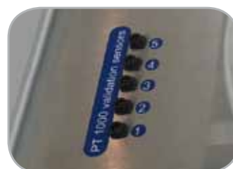
PT1000 temperature validation ports
