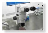
Having an integrated stereomicroscope in the work chamber makes it possible to keep the culture dishes at the right temperature at all times while observation and manipulation is being carried out.
