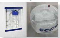
Gas outlet is located on the table surface. The plastic cover encloses the humidified gas effectively and creates a small incubator environment.
