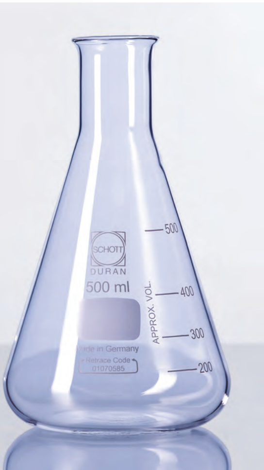
Borosilicate glass 3.3 Erlenmeyer flask
