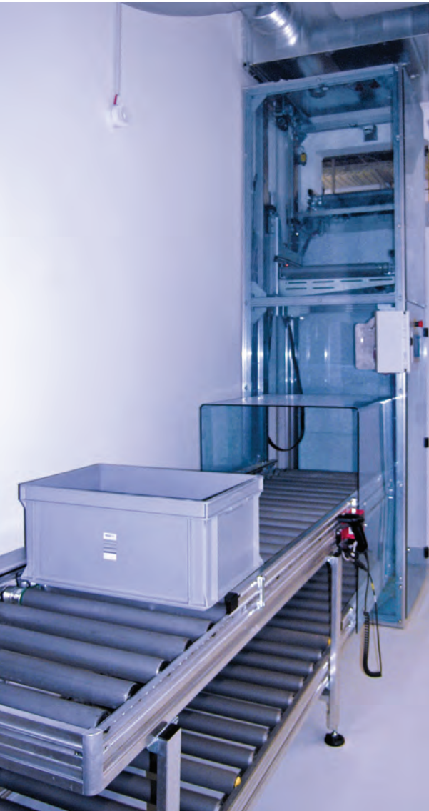
Outfeed side of a transport box system
