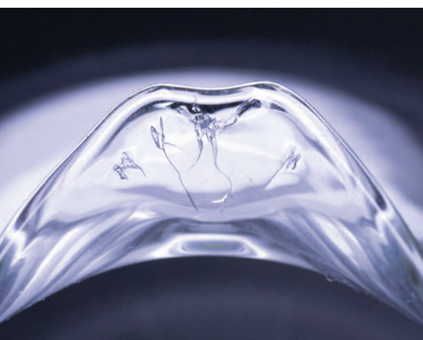
Cracks in the spout of a laboratory beaker
