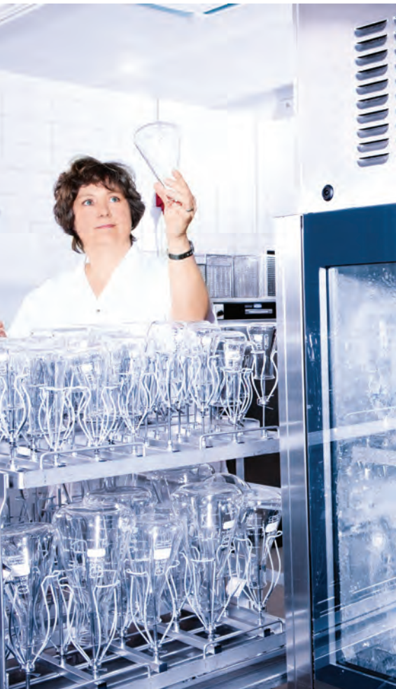
Visual inspection of laboratory glassware following automated reprocessing
