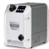
VACUU-PURE 10C Screw pump 9 m 3 /h, 5 x 10 -3 mbar Vacuum connection: Small flange DN 25
