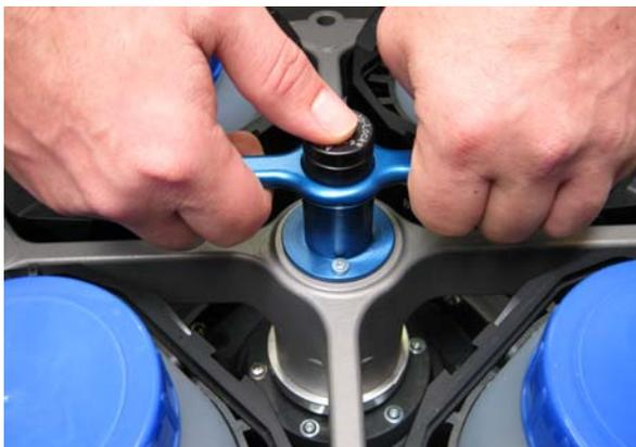
**Figure 2.** Removing the Rotor
