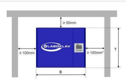
All dimensions are minimum dimensions and should not be reduced to safe the heating power emission without problems.
