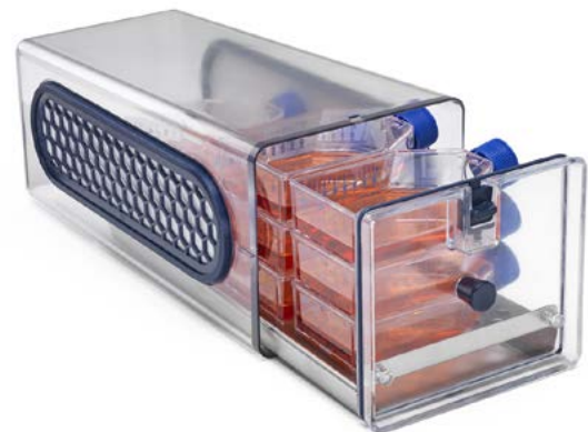
Figure 2: Each Cell Locker Chamber features dual 0.2 µm membrane filters which permit air exchange but restrict microorganisms from entering or exiting. The chamber will hold nine T-75 flasks or up to twenty-eight micro-well plates.
