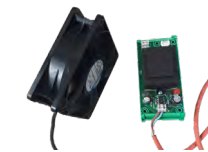
Explosion-proof fan with ATEX power cable and energy limiting power supply.
