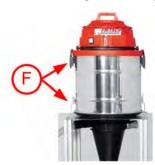
The exhaust system can be disassembled and cleaned after opening the clips (F). To open and clean the cyclone separator, 4 screws in the inner part of the base must be loosened.
