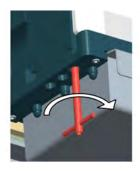
At this time, it is not possible to switch on the Universal Cutting Mill. To switch it on, the safety lock (11) must be activated by turning the triangular key to the left, the closing lid (6) must be closed and the latch clamp (13) in locked position.
