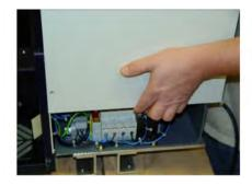
Two U-profiles (12) are mounted on the bottom of the device. Insert the 4 screws provided through the bore holes in the U-profiles (12) and screw them tightly to the stand or table. Other screws with the same diameter can also be used.
