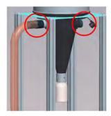
Attach one end of the connection hose (28) with the rubber sleeve (29) to the adapter (27) and the other end to the cyclone separator (30).
