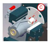
Push the rotor (3) onto the rotor holder. Turn it clockwise until it engages in the 4 driving pins (C) on the back. (The control switch (19) must be at AUTO)
