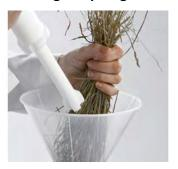
The plunger has 2 different sides for feeding the sample material in the funnel to the grinding chamber. On the one hand, the smooth, round side is suitable for finer material. On the other hand, the cross-shaped, thinner side is suitable for long, fibrous material, like straw.
