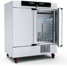
Stainless steel W.-St. 1.4301 (ASTM 304), deep drawn Chamber
