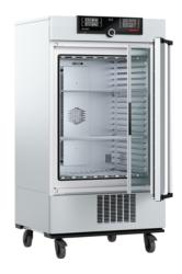
Chamber Stainless steel W.-St. 1.4301 (ASTM 304), deep drawn
