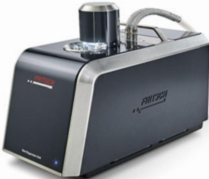
**Transparent hoses** made of silicone with especially smooth interior surfaces are barely susceptible to deposits and make soiling or blockages directly visible.
