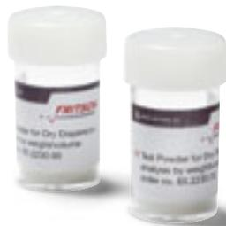
Reference material for inspecting the measuring system
