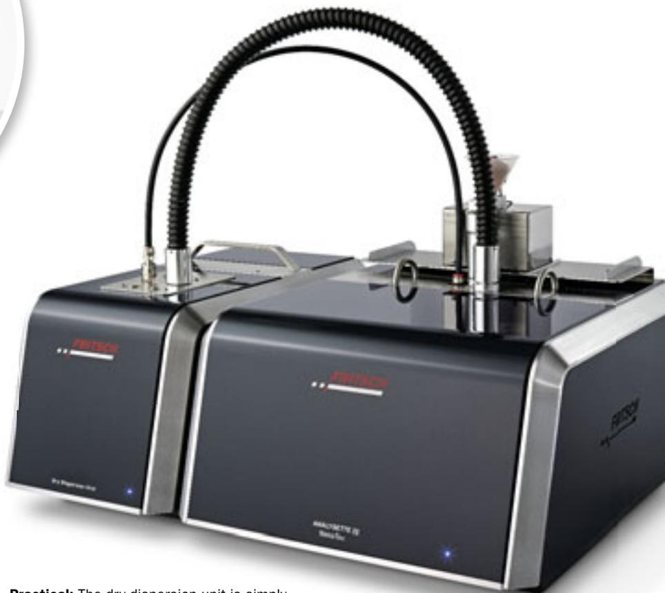
**Practical:** The dry dispersion unit is simply connected to the measuring unit as a module
