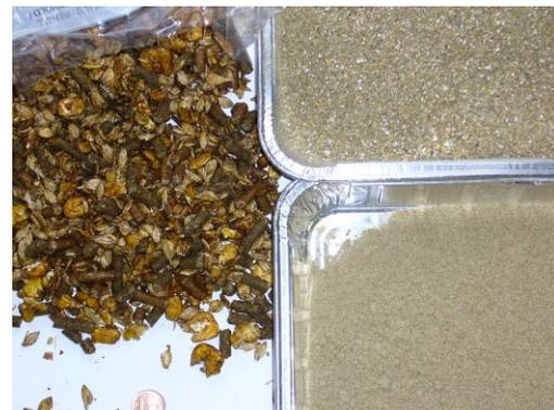
Upper photo to the right: a glance into the opened collecting pan of the mill, the sample put through the 2 mm sieve. Visually the result is still clearly inhomogeneous. For the creation of a smaller mixed sample, for the second step of the comminution, by all means a sufficient mixing and exact sample division is to be kept in mind. For the division of the sample we recommend the [Rotary Cone Sample Divider LABORETTE 27](#).
